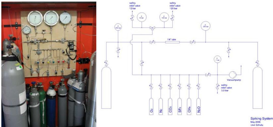
**Figure 2: Spiking system for adjustment of mixing ratios in natural air samples**
